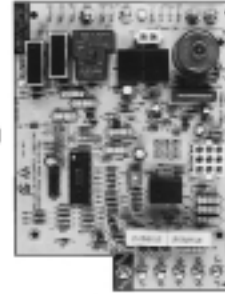
INTEGRATED FURNACE CONTROL
